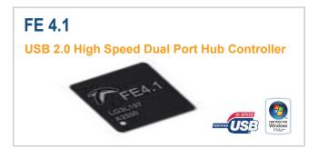
As all other hub controller series products from Terminus, the high quality of FE 4.1 is guaranteed by Design-For-Testing with comprehensive scan chains and Built-In-Self-Test modes which could exercise all High-, Full- and Low-Speed Analog Front End (AFE) components during the packaging and testing stages.
