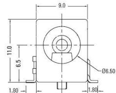
**CN12 Power Supply Connector (optional/internal)**
