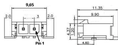
**CN12A Power Supply Connector (optional/internal)**
