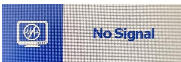
If no valid video signal can be detected the board is powered down and the following message will be displayed
